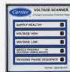
2. VOLTAGE SCANNER (3-phase compressor protection relay):- It is a stand-alone microcontroller based protection device which is to provide electrical safety of 3-phase compressor and fan motor from abnormal voltage conditions in field. It provides electrical protection against Phase reversal, Phase Loss, Phase to Phase voltage unbalance and Over & Under voltage.
